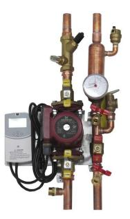
The commercial pump station can be used in situations where the closed loop system has higher head and flow requirements. This pump station can be used with up to 10 x AP-30 collectors (2 banks of 5 AP-30).
